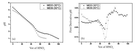
FIGURE 2. Titration of 0.10 M AHM with 1.0 M HNO<sub>3</sub> at different temperature for (a) pH and (b) pH first derivative
