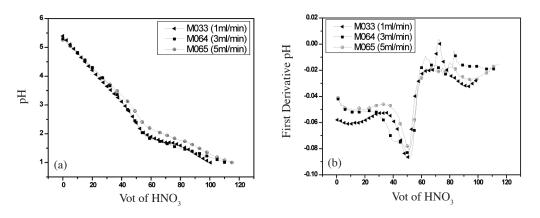
FIGURE 4. Titration curve and derivative of 0.10M AHM with 1.0 M  $\text{HNO}_3$  at different rate of addition for (a) pH and (b) pH first derivative
