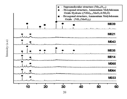
FIGURE 1. XRD patterns of synthesized samples
