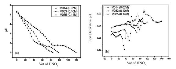
FIGURE 3. Titration of AHM at different concentration with 1.0 M HNO<sub>3</sub> at 1mL/min for (a) pH and (b) pH first derivative
